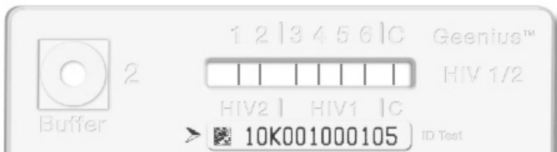
The Geenius™ HIV 1/2 Supplemental Assay cassette contains a Control band (C) and six (6) test lines which are numbered on the cassette corresponding to the following:
